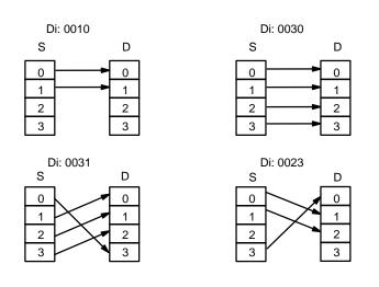
ER: At least one of the rightmost three digits of Di is not between 0 and 3. Indirectly addressed DM word is non-existent. (Content of \*DM word is not BCD, or the DM area boundary has been exceeded.)
